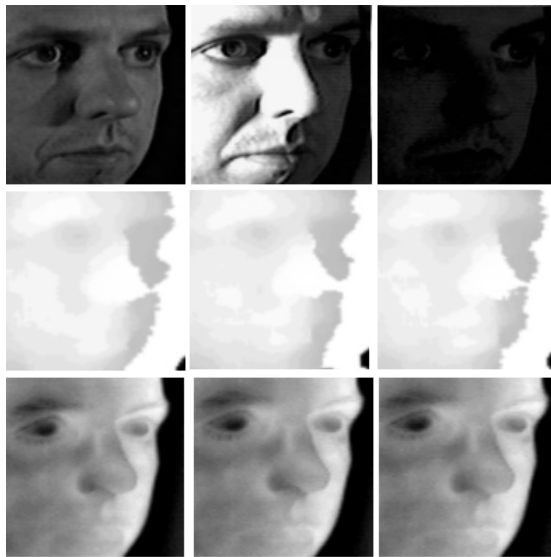
Figure 10: An example of the LM2 lighting variations for the left side pose VIS (first row) depth (second row) LWIR (third row) images. From left to right: Front-lit, side-lit and low-light
