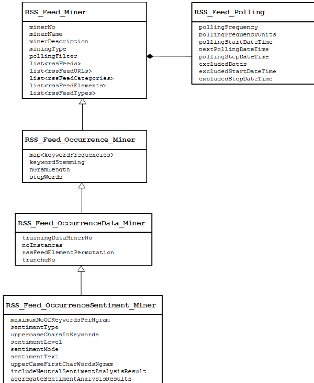
Figure 4.7: UML class diagram of visualRSS's class hierarchy for case study two, and its extension for our classification and sentiment analysis work (methods have been edited for clarity): cf. case study three .
