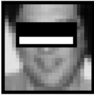
Figure 2.8. The upper face region represented as a Haar-like feature. Source: Viola & Jones (2001).
