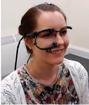
Figure 2.1. Participant wearing the Positive Science head-mounted eye tracker.
