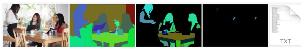
Figure 4.6: PSPNet’s 3 level of abstraction: (i) objects (level 1), (ii) object parts (level 2), and (iii) parts of object parts (level 3). The network starts with a photograph and outputs a text file containing the probabilities of objects and/or object parts.
