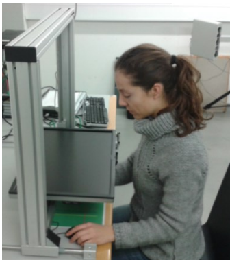
Fig.2. Experimental setup for the localization task. The right hand is lying in upright position on the table while being covered by the screen and thereby hidden from the participant's view. The localization of the right hand's landmarks was done by directing the mouse cursor (with the left hand) to the corresponding location on the screen. Participants were asked to place the mouse pointer on the screen directly above where it felt like the tip or knuckle of their finger was positioned.
