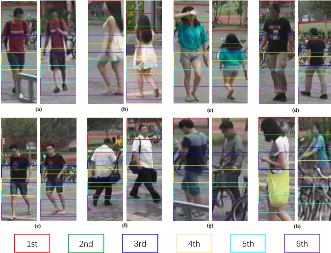
Fig. 9. The vertical alignment module can detect body parts robustly under a vast majority of circumstances, including moderate (a, b) or even severe (c, d) part misalignment, dramatic pose variations (e, f), and occlusion (g). However, the vertical alignment module may fail in cases where complex occlusion or a part missing problem exist (h). Best viewed in color.
