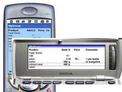
Figure 4. Access to retail m-services via cellular wireless mobile devices: user authentication (left) and shopping list editing (right) on wireless enabled personal digital assistant and cellular mobile telephone (both Java 2 Micro Edition capable).
