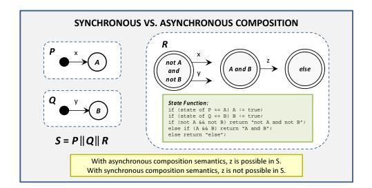
Figure 2.1: Synchronous and Asynchronous Composition
