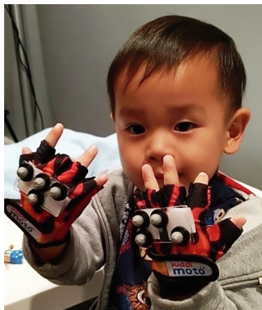
Fig. 1. A participant wearing the motion capture gloves with the two distinct plates of optical markers for the left and right hands.
