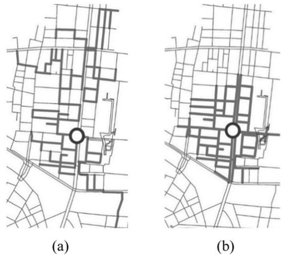
Fig. 2 Illustrative examples of sub-networks with a an irregular, complex network ( K_{NT}(Z)=0.3 ), and b the most compact network ( K_{NT}(C(Z))=1.0 )
