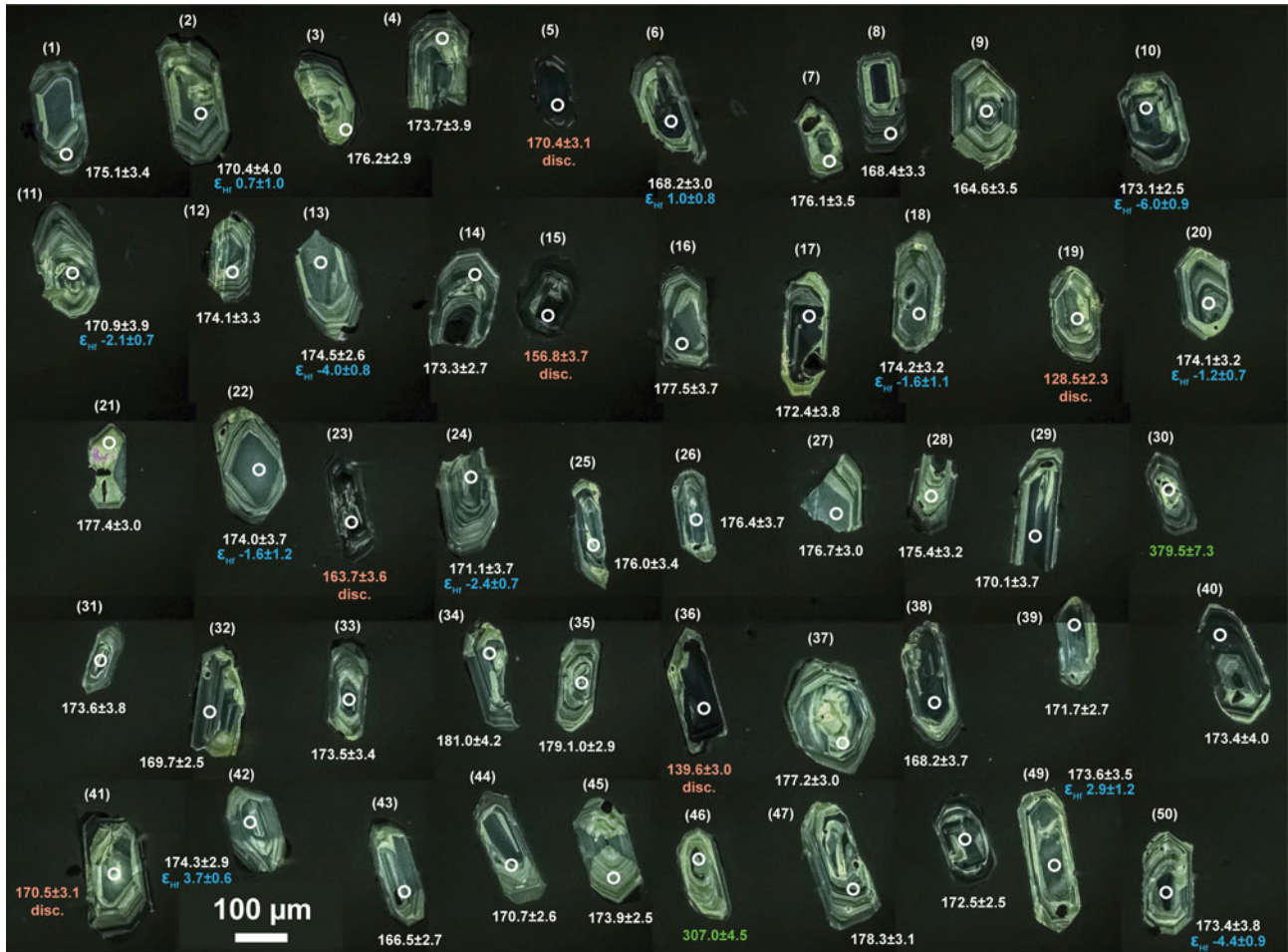
Figure 5. Cathodoluminescence images and U-Pb dates of the 50 zircon grains analysed from sample SIA (SI = Sif Island). Red text indicates discordant ages, and the two Palaeozoic inherited cores are highlighted using green text. Also shown are the \epsilon_{Hf} values (blue text).
