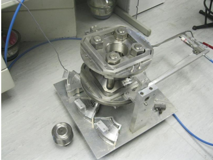
Figure 7.5. Image taken during the 2012 experiment showing assembled P-E cell before mounting in cradle.
