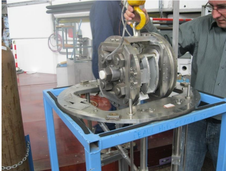
Figure 7.6. Image taken during the 2012 experiment showing the P-E cell being lowered into its cradle.
