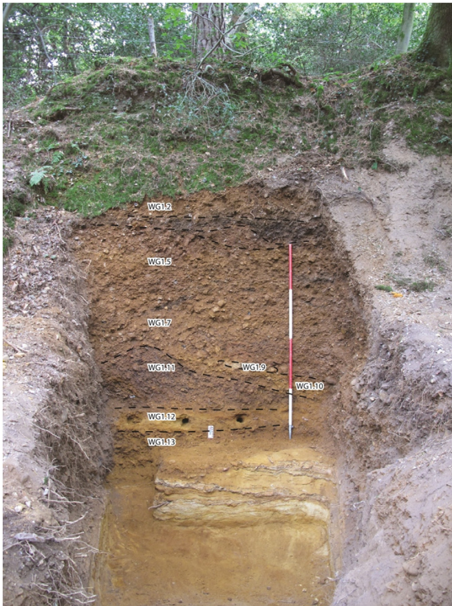
Fig. 21. Section 1 excavated at Wood Green Gravel Pit at SU 1719 1700 around 2015. From Egberts et al. (2019, 2020). The black sampling holes show the location of OSL samples WG1E01, WG1E02 and WG1E03, whose results are given in Table 4. Photograph: Ella Egberts.
