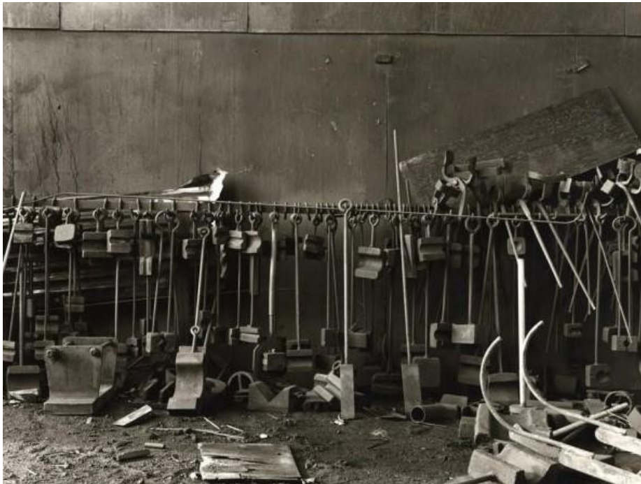
Fig. 18 Blacksmiths' tools. Blacksmiths' tools in the forge. Each craftsman designs and makes his own tools Bruce Rae, Amber associate photographer, Photograph, Circa 1980
