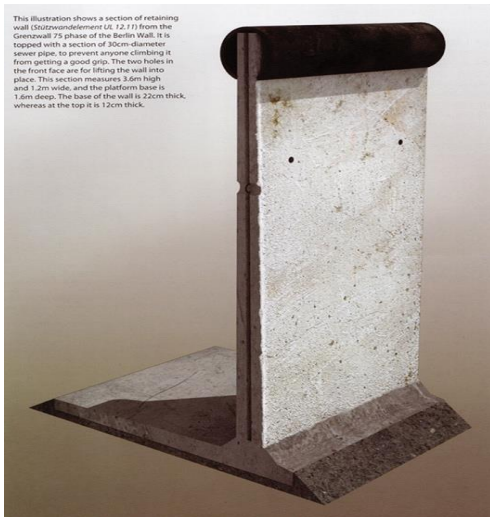
Diagram of Grenzmauer 75 (4), Wall segment (frontline wall) topped by sewer pipe: 3.6m high, 1.2m wide, the platform base is 1.6m deep, the base is 22cm thick, the top is 12 cm thick.
