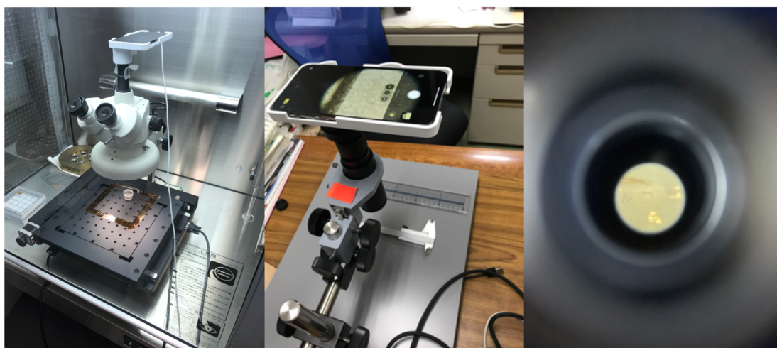
Figure 3.1: Adapting the LabCam® and iPhone Pro Max 12 into the ISAS CLOXS system. Left: Clean bench set up to start single-operator imaging and analysis. Note the LabCam® mount, and 50mm traverse motorised xy stage, 100mm traverse stage and joystick controls. Centre: Hozon Co. Ltd. microscope and LabCam® mounted with iPhone Pro Max 12 for calibration. Right: Looking remotely ‘down the hole’ of the iPhone Pro Max 12 at a magnified block particle fragment in the aerogel.
