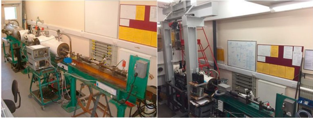
Figure 3.6: Two-stage gas gun set up at University of Kent Canterbury; Left, horizontal gun; Right, with vertical axis gun framework emplaced. Horizontal barrel length is c. 5 metres. (see Hibbert 2017 [116] and Burchell 1999 [117]).
