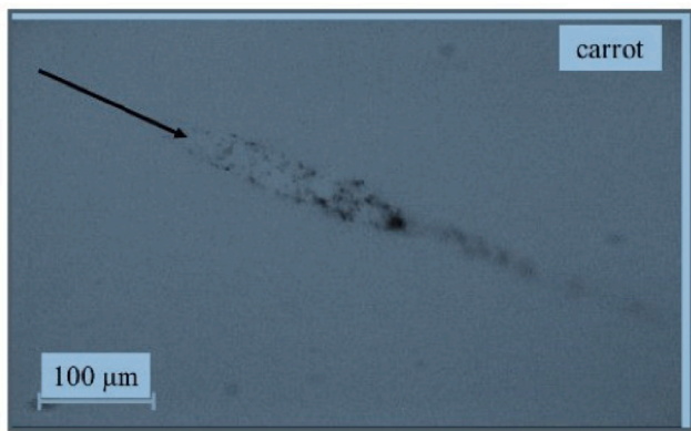
Fig. 5. A ‘carrot’ shaped track of a hypervelocity impactor in the Tanpopo silica aerogel panel returned from the International Space Station. The arrow indicates an impact direction.
