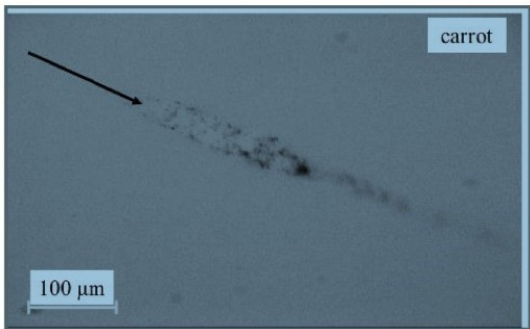
Figure 2.5: A 'carrot' shaped track of a hypervelocity impactor in the Tanpopo silica aerogel panel returned from the International Space Station. The arrow indicates the impact direction. Viewed from above, i.e. the track is roughly parallel to the surface.
