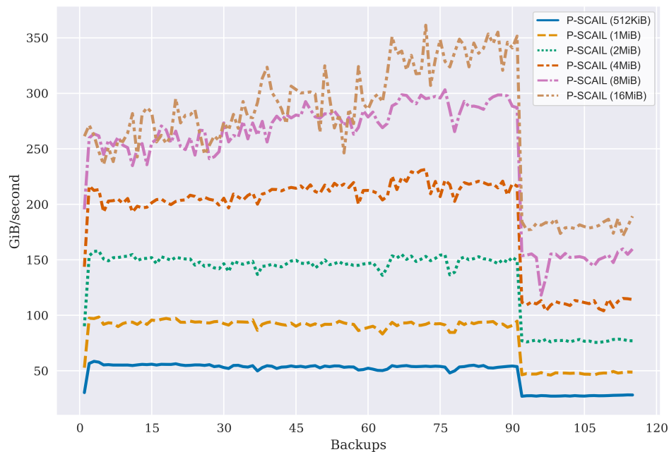
Figure 6.19: FSL Dataset: Multiprocessor Throughput Performance of P-SCAIL with Different Segment Sizes. Larger segment sizes result in higher throughput. A dropoff in throughput after 95 backups is caused by reduced logical data submitted for backup, which can be observed in Figure 6.20.
